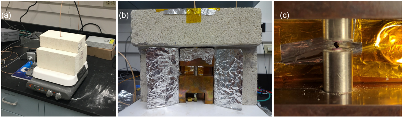
FIG. 5. Custom-built high temperature RUS setup. Panel (a) shows the entire setup covered by insulating firebricks. In panel (b), one of the firebricks has been removed to give a better view of the copper mount. Panel (c) shows a sample being mounted on its corners between two piezoelectric transducers.
