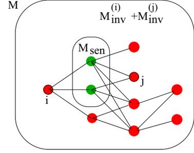
FIG. 4. The sensitivity set  $M_{\text{sen}}$  of the conductance  $\mathbf{G}_{ij} = 0$ .
