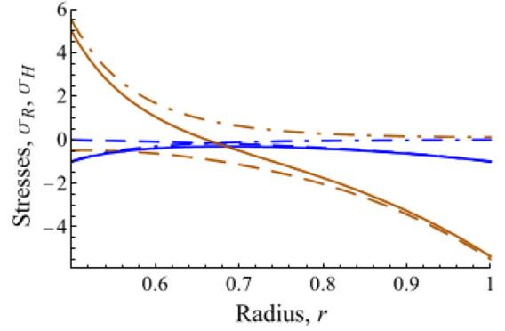
FIG. 2. The radial (blue curves,  $0 < y < 1$ ) and hoop stresses (brown curves to large positive and negative values) are plotted against radius for a material as anisotropic as graphene, for internal pressure  $P_a = 0$ , external pressure  $P_b = 1$  (dashed curves), for  $P_a = 1$ ,  $P_b = 0$  (chain-dotted curves), and for hydrostatic pressure  $P_a = 1$ ,  $P_b = 1$  (solid curves). The outer diameter is unity, and the inner diameter is  $\frac{1}{2}$ .
