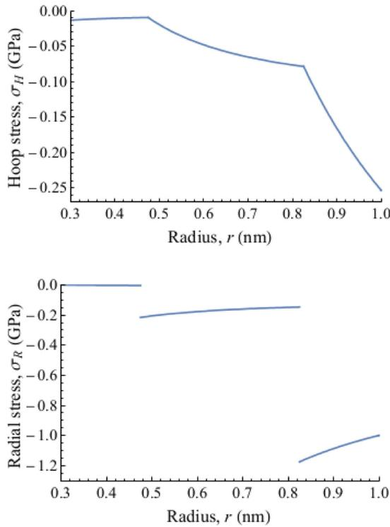
FIG. 4. The hoop (top graph) and the radial (bottom graph) stresses in the 3D material are plotted against radius, from the outer surface of the outer tube to the inner bore of the inner tube.
