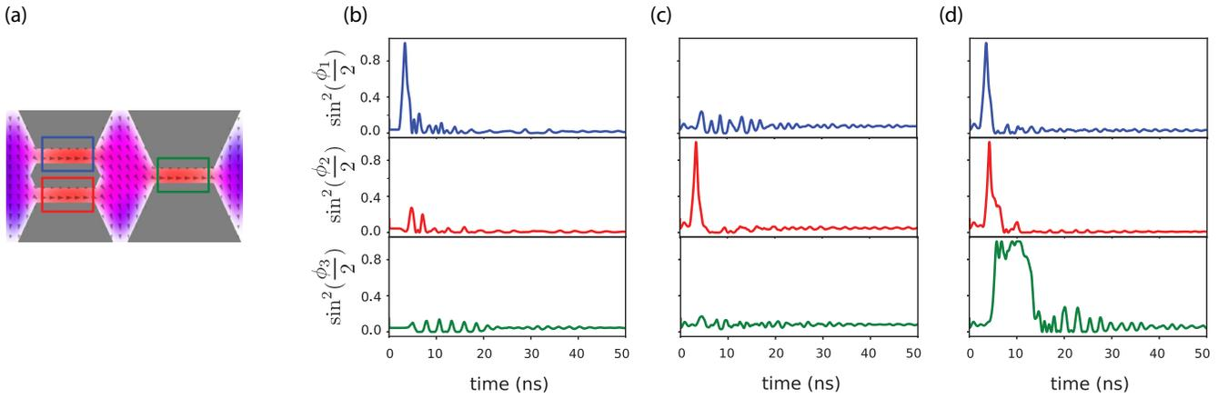
FIG. 7. (a) Top view of a “two-to-one” neural network building block. (b) Current input only in the first of the input layer neurons (blue), the output neuron (green) does not spike. (c) Current input only in the second of the input layer neurons (red), the output neuron does not spike. (d) When both input neurons spike, the energies of output spin waves sum up and make the output layer neuron spike.
