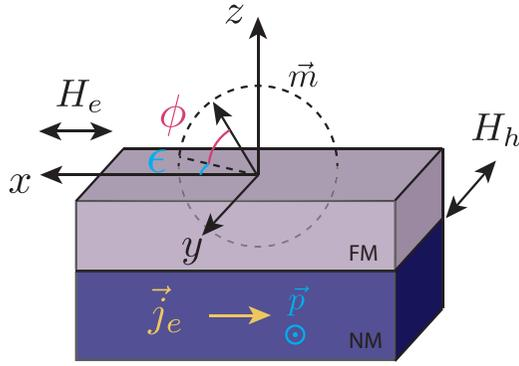
FIG. 1. Schematic of an easy-plane spin Hall nano-oscillator. The bottom layer is a normal heavy metal (NM) that polarizes the electrical current  $j_e$  in spin. The top layer is a ferromagnet (FM) with a net easy plane (the  $xz$ -plane) perpendicular to the polarization  $\vec{p}$  of the injected spins. The magnetization  $\vec{m}$  precesses in the  $xz$ -plane with phase  $\phi$  and small out-of-plane tilt  $\epsilon$ .
