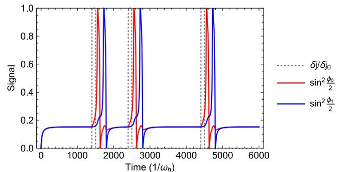
FIG. 3. Spiking dynamics of the in-plane phase for the neuronal spins  $\phi_0$  and  $\phi_1$ . The system is held close to threshold until a small current pulse is applied to  $\phi_0$  during a time interval during indicated by the dotted lines. This causes a phase spike for  $\phi_0$  (red curve). A short time later,  $\phi_1$  spikes due to excitations from the  $\phi_0$  spike pushing it over its threshold (blue curve). The process is then repeated multiple times with different intervals.
