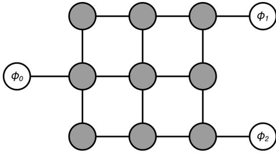
FIG. 9. Lattice topology of the macrospin fan-out simulation. The “upstream” neuron  $\phi_0$  generates a spike after being given a perturbative current  $j$  on top of the static current  $j$ . The “downstream” neurons  $\phi_1$  and  $\phi_2$  both spike in response, as a consequence of spin excitations mediated by the  $3 \times 3$  lattice.
