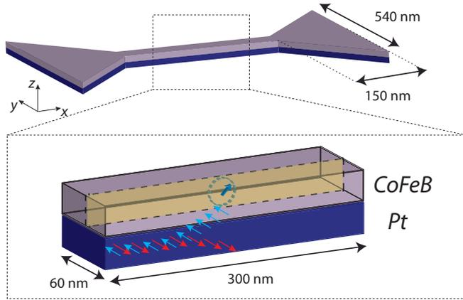
FIG. 4. Geometry for micromagnetic simulations. The bottom layer is normal heavy metal such as Pt and the top layer is a 2 nm thick CoFeB. The dark blue arrow shows large in plane (yellow)  $2\pi$  precessions of the top layer magnetization.
