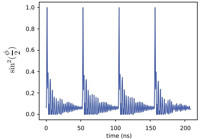
FIG. 6. Normalized tunneling magnetoresistance of the nanoconstriction easy-plane SHNO. Current pulses with density  $j = 2.5 \times 10^{10}$  A/m<sup>2</sup> are applied over 2 ns time intervals spaced by 50 ns.
