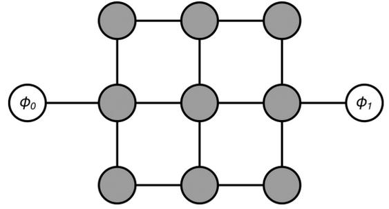
FIG. 2. Lattice topology of the macrospin simulation. Each circle represents a macrospin. White circles ( $\phi_0$  and  $\phi_1$ ) are neuronal macrospins with easy-plane anisotropy and other relevant interactions; gray circles are synaptic macrospins. Connections between macrospins indicate the presence of an exchange interaction.
