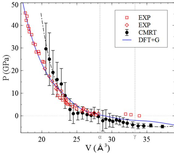
FIG. 2. The  $P$ - $V$  data obtained from CMRT are compared against experiments [32,33]. DFT + G at  $U = 6$  eV with SOC [23] is also included as the 0 K pressure reference. Error bars of CMRT pressure are derived from those in total energy calculation, see Supplemental Material Ref. [34].
