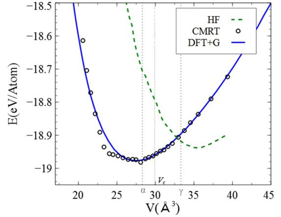
FIG. 1.  $E$ - $V$  curves on fcc Ce calculated with nonmagnetic HF, DFT + G with  $U = 6$  eV (upper right panel of Fig. 1 in Ref [23]), and CMRT. Taking CMRT energy as the reference, arbitrary vertical energy shift are applied to HF and DFT + G for a best comparison with CMRT.
