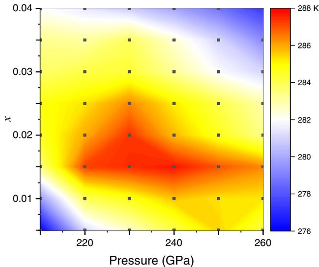
FIG. 4. Dependence of  $T_c$  on doping level and pressure for  $\text{LaH}_{10-x}\text{N}_x$  with  $\mu^* = 0.10$ . The black dots represent the calculated data grid.
