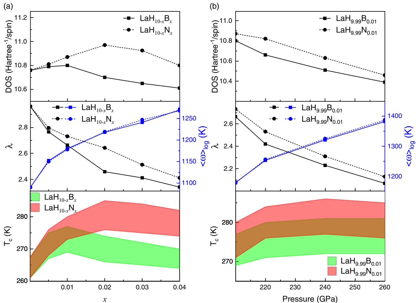
FIG. 3. (a) DOS,  $\lambda$ ,  $\langle\omega\rangle_{\log}$ , and  $T_c$  of  $\text{LaH}_{10-x}\text{B}_x$  and  $\text{LaH}_{10-x}\text{N}_x$  with different doping levels at 210 GPa. (b) DOS,  $\lambda$ ,  $\langle\omega\rangle_{\log}$ , and  $T_c$  of  $\text{LaH}_{9.99}\text{B}_{0.01}$  and  $\text{LaH}_{9.99}\text{N}_{0.01}$  at different pressures. For each  $T_c$  curve, the upper and lower bounds are obtained by choosing  $\mu^* = 0.10$  and 0.11, respectively.
