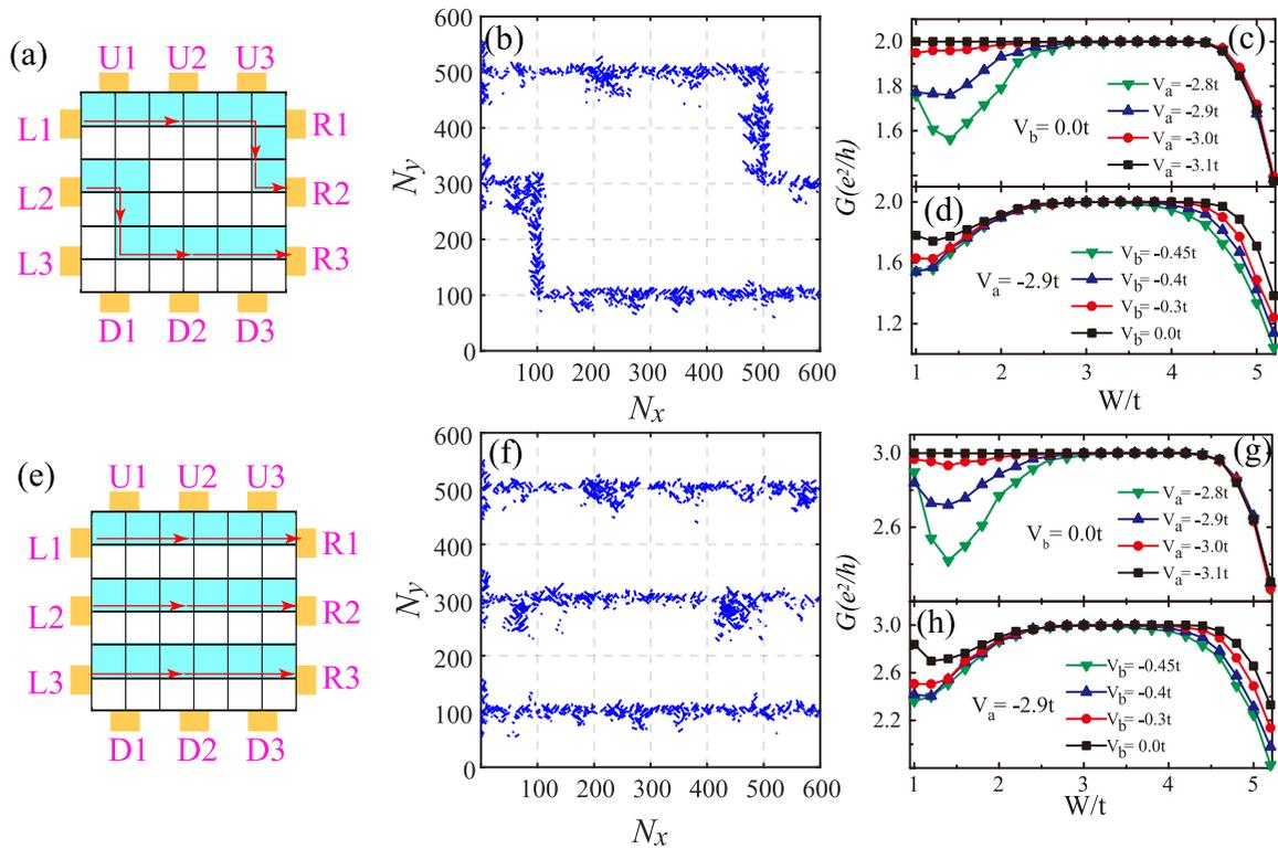
FIG. 3. [(a),(e)] Schematic of programmable circuit devices, which have two and three chiral interface channels, respectively. [(b),(f)] Local current density distribution corresponding to cases [(a),(e)] with gate voltage  $V_a = -2.8t$ ,  $V_b = 0$  and disorder strength  $W = 3.5t$ . [(c),(d)] and [(g),(h)] Conductances  $G$  vs  $W$  for different  $V_a$  and  $V_b$ , respectively.
