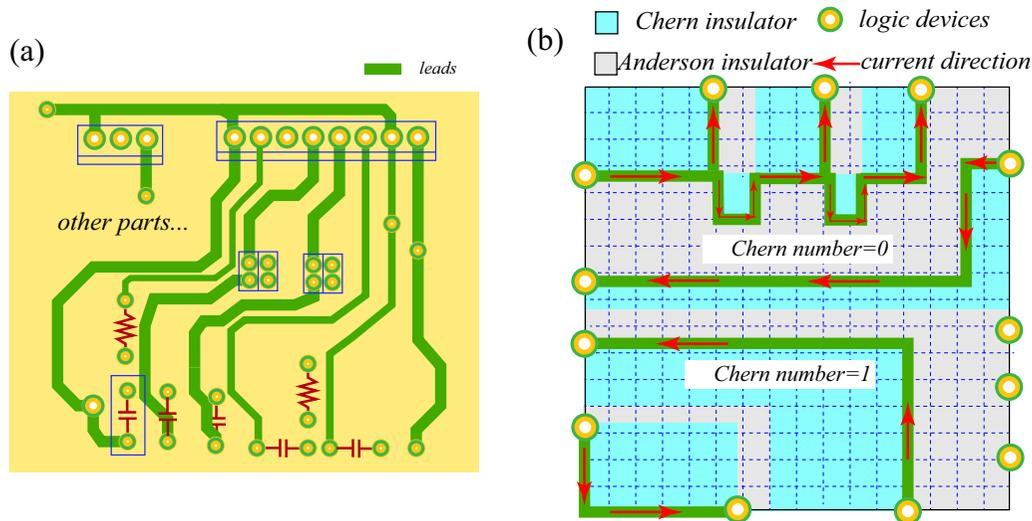
FIG. 1. (a) Schematic plot of a conventional printed circuit board. The orange areas are the background. The solid green lines are the wires and the logic devices are marked in yellow circles. (b) Schematic plot of a programmable integrated circuit based on disordered CIs. The central region is divided into several cyan and gray blocks. The red arrows denote the current directions.
