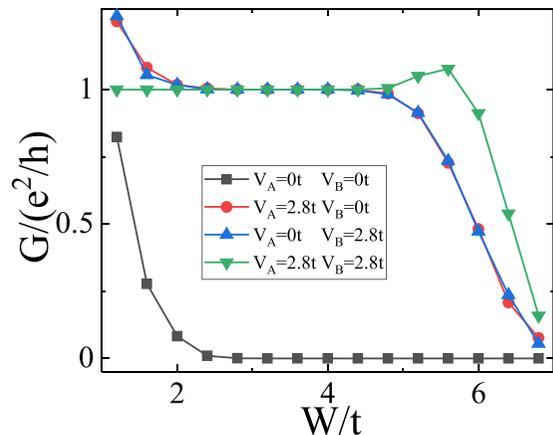
FIG. 6. Differential conductances  $G$  versus disorder strength  $W$  for OR gate.
