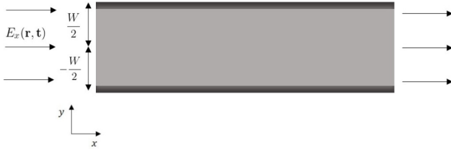
FIG. 1. Two-dimensional Fermi liquid confined in a slab setup. The width of the slab is W and the electric field is applied in the horizontal direction. The darker areas in the sample are the walls that we will describe through the collision integral I_{\text{bd}} in the transport equation
