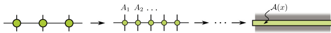
FIG. 3. The continuum limit of discrete matrix product operators (MPO) gives rise to a continuous matrix product operator (cMPO). Both are characterized by finite-dimensional matrices A_i [respectively \mathcal{A}(x) ], indexed by a discrete (respectively continuous) position label, whose entries are operators acting on the corresponding lattice site i (respectively point x on the line).
