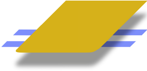
FIG. 1. Schematic illustration of a contact (orange) side-attached to a chiral (not terminating in the contact) two-channel edge (blue). The contact is connected to an external circuit and coupled to the edge modes through tunneling bridges.
