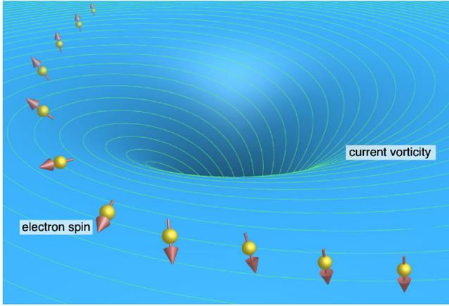
FIG. 1. Schematic figure of spin-vorticity coupling. The red arrow with a yellow sphere denotes the conduction electron spin, which is scattered by the current vorticity due to spin-vorticity coupling.
