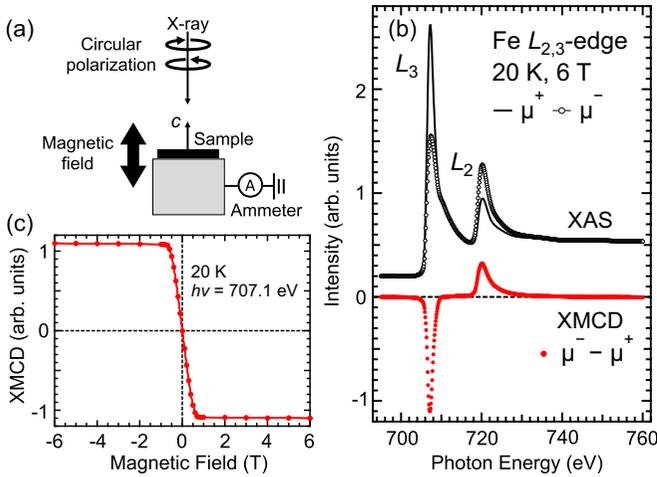
FIG. 2. (a) The experimental geometry of XAS/XMCD measurements in total electron yield (TEY) mode. See method part for details. (b) The Fe  $L_{2,3}$ -edge XAS and XMCD spectra at 20 K under 6 T. The  $\mu^+$  ( $\mu^-$ ) denotes the XAS absorption intensity for parallel (antiparallel) alignment of the photon helicity and the sample magnetization direction. (c) The magnetic field dependence of the XMCD intensity of Fe  $L_3$  (707.1 eV) at the photon energy of the XMCD peak.
