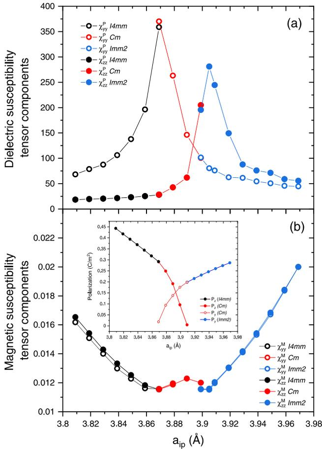
FIG. 3. Dielectric (a) and magnetic susceptibility (b) tensor components of epitaxial (001) SBMO films as a function of  $a_{ip}$  in  $14mm$ ,  $Cm$ , and  $Immm2$  states. The inset in (b) shows the polarization values of SBMO films as a function of  $a_{ip}$ .
