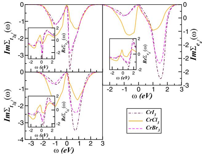
FIG. 4. Orbital-resolved self-energy imaginary (main panels) and real (insets) parts of  $\text{CrX}_3$  bulk crystals, showing their chemical evolution for fixed  $U_{t_{2g}^1} = 2.75$  eV,  $U_{t_{2g}^2} = U_{e_g} = 4.0$  eV, and  $J_H = 0.85$  eV values. A particular feature to be seen is the clearly visible particle-hole asymmetry and the strong frequency dependence of the self-energy real parts within the Mott localized  $\text{CrI}_3$  and  $\text{CrBr}_3$  systems.
