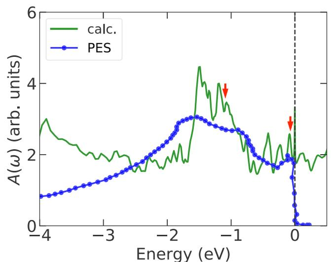
FIG. 3. Electronic density of states of  $\text{PuIn}_3$ . The calculated and experimental data are represented by solid thick line and circles, respectively. The calculated data are multiplied by the Fermi-Dirac distribution function. The experimental data are extracted from Ref. [28] at photon energy of 40.8 eV (blue circles).
