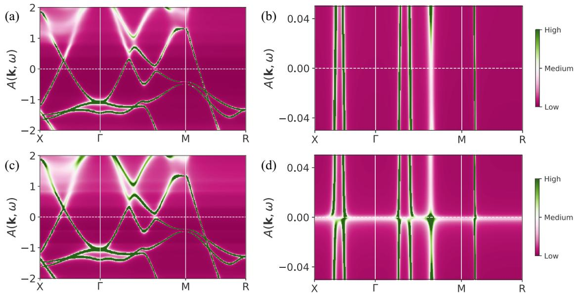
FIG. 2. Momentum-resolved spectral functions  $A(\mathbf{k}, \omega)$  of  $\text{PuIn}_3$  as a function of temperature under ambient pressure obtained by DFT + DMFT calculations. (a) 580 K. (c) 14.5 K. An enlarged view of panel (b) 580 K and (d) 14.5 K in the energy window  $\omega \in [-0.05, 0.05]$  eV. In these panels, the horizontal lines denote the Fermi level.
