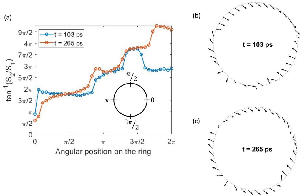
FIG. 5. (a) The direction pointed by the linearly polarized Stokes vector  $S_1\hat{x} + S_2\hat{y}$  around the ring at two time instances. The angle  $\tan^{-1}(S_2/S_1)$  has been unwrapped in the range  $[0, 6\pi]$ . Parts (b) and (c) show the linearly polarized Stokes vector in the ring at  $t = 103$  and  $265$  ps, respectively.
