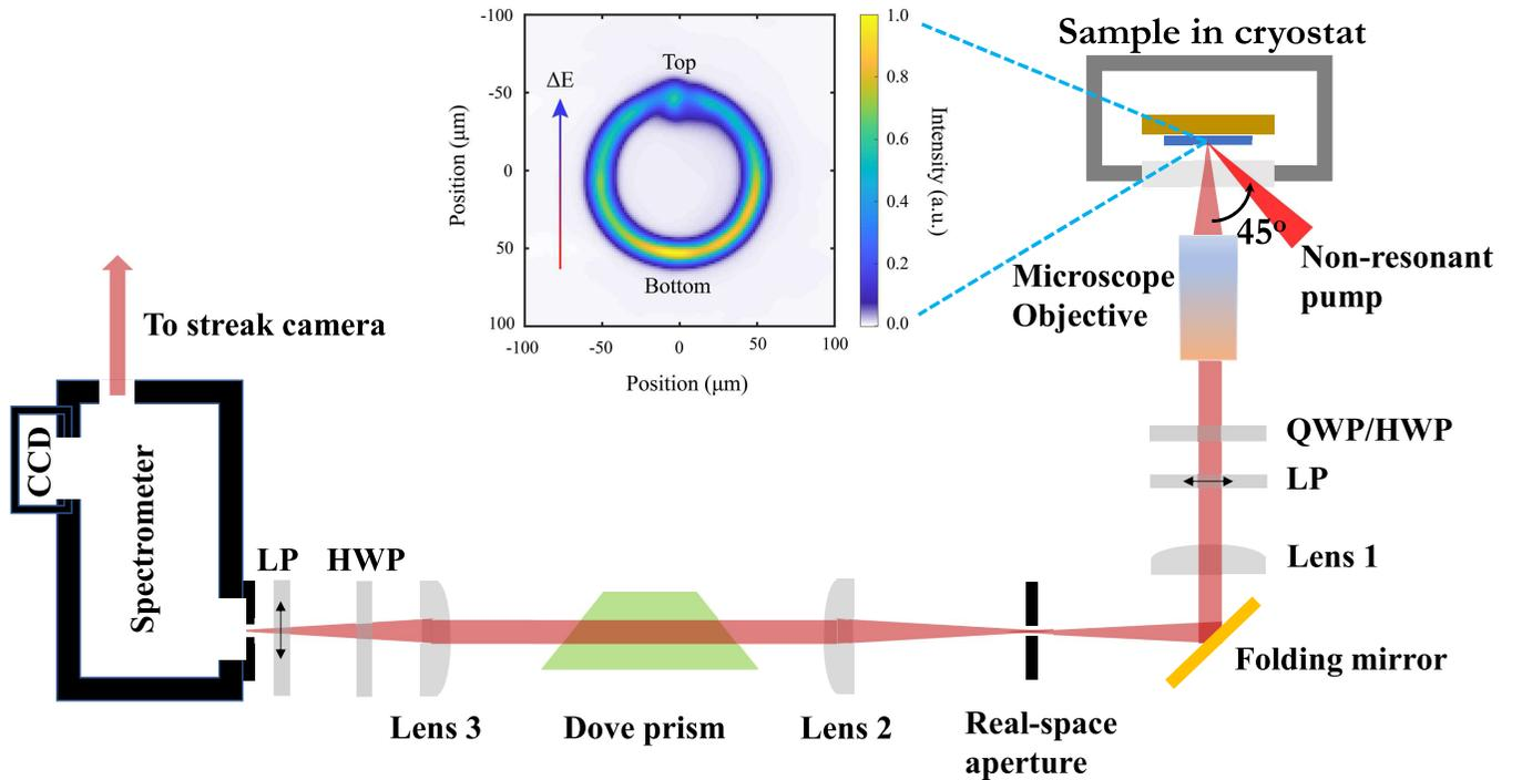
FIG. 1. Schematic of the experimental setup. The inset shows a time-integrated image of the photoluminescence from the ring microcavity also showing the direction of the cavity gradient  $\Delta E$ . QWP: quarter waveplate, HWP: half-waveplate, LP: linear polarizer.
