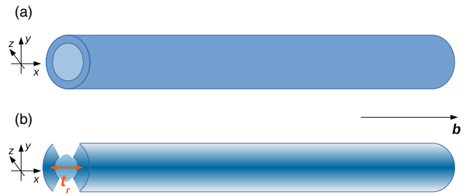
FIG. 1. Electronic (charge and spin) densities along a 1D column. (a) Homogeneous density on a surface of a cylinder, a tube. This is the case realized in, e.g., carbon nanotube and has been solved in Ref. [13]. (b) The case of more complex orbital when electrons reside only on a section of a tube, moreover with a density that is not uniformly distributed inside the occupied zone. In the case (b) we can define two parts connected through their respective orbital's hybridization t_r . In both cases, the 1D column is along the b axis of a quasi-1D crystal. Moreover, we define a local system of coordinates (x, y, z) which is used to integrate the interaction potential. Please note that in both cases we give a density that comes from an electron wave function in a given conduction band (eigenorbital) \psi_{L/R,\alpha}(\vec{r}) in a vicinity of the Fermi level.
