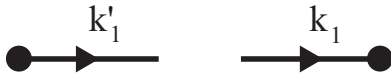
FIG. 13. External vertices represent annihilation operators with wave vector k'_1 or creation operators with wave vector k_1 .
