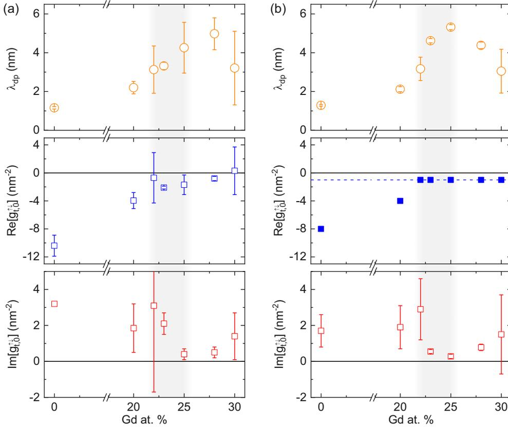
FIG. 16. Comparison of modeling results with (a) free  $\text{Re}[g_{t,0}^{\uparrow\downarrow}]$  and (b) fixed  $\text{Re}[g_{t,0}^{\uparrow\downarrow}]$ . The shaded region indicates the window of composition corresponding to magnetic compensation.
