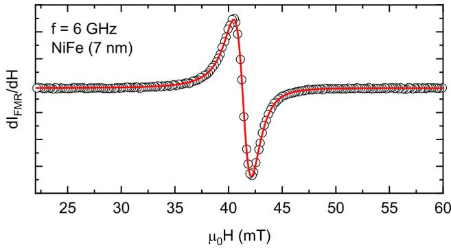
FIG. 9. FMR spectrum of  $\text{Ni}_{80}\text{Fe}_{20}(7)/\text{Cu}(4)$  at 6 GHz. The red curve represents the fit using Eq. (A1).
