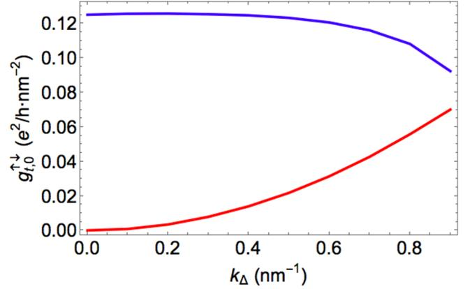
FIG. 15. Interfacial transmitted mixing conductance versus the exchange splitting  $k_\Delta$ .  $\text{Re}[g_{t,0}^{\uparrow\downarrow}]$  in blue and  $\text{Im}[g_{t,0}^{\uparrow\downarrow}]$  in red.
