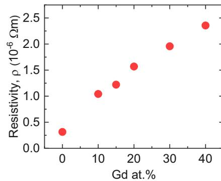
FIG. 13. Resistivity  $\rho$  with varying Gd at. % for SiO<sub>x</sub>(thermally oxidized)/Co<sub>100-x</sub>Gd<sub>x</sub>(10)/TiO<sub>x</sub>(3) (unit: nm). The resistivities of intermediate compositions between  $x = 20$  and 30 are derived via linear interpolation.
