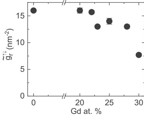
FIG. 11. Composition dependence of the renormalized reflected mixing conductance  $\tilde{g}_r^{\uparrow\downarrow}$  at the Cu/Co<sub>100-x</sub>Gd<sub>x</sub> interface with the Co<sub>100-x</sub>Gd<sub>x</sub> spin sink thickness  $d \gg \lambda_{dp}$ .
