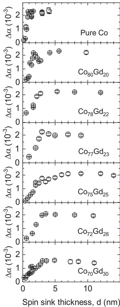
FIG. 4. Nonlocal damping enhancement  $\Delta\alpha$  versus spin sink thickness  $d$  for CoGd spin sinks with different compositions.
