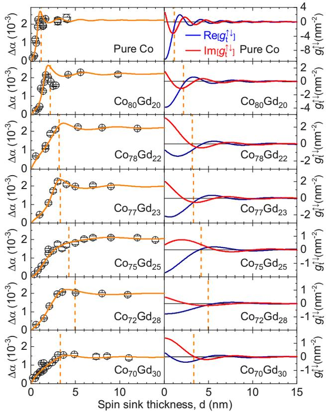
FIG. 6. Left column: Spin sink thickness dependence of nonlocal damping enhancement  $\Delta\alpha$ . The solid curve indicates the fit using the modified drift-diffusion model. Right column: The real and imaginary parts of the transmitted spin-mixing conductance  $g_{t,0}^{\uparrow\downarrow}$  derived from the fit. The vertical dashed line indicates the spin dephasing length  $\lambda_{\text{dp}}$ .
