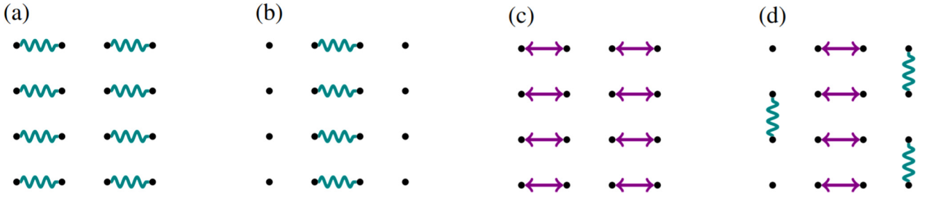
FIG. 4. Quantum circuit elements required to implement one layer of the EHV or NP ansatz for a single spin-type. Circuit layers go from (a) to (d), with (c) and (d) repeated thrice more to complete the swap network. Wavy green lines are the number-preserving unitaries U_{\text{NP}} . Purple arrows are FSWAP gates, with (c) representing U_L and (d) representing U_R implemented in parallel with vertical hopping terms. In our implementation, the (b) layer is moved to the end, allowing the horizontal hopping terms in (a) and (b) to be combined with the FSWAP gates in (c) and (d), respectively.
