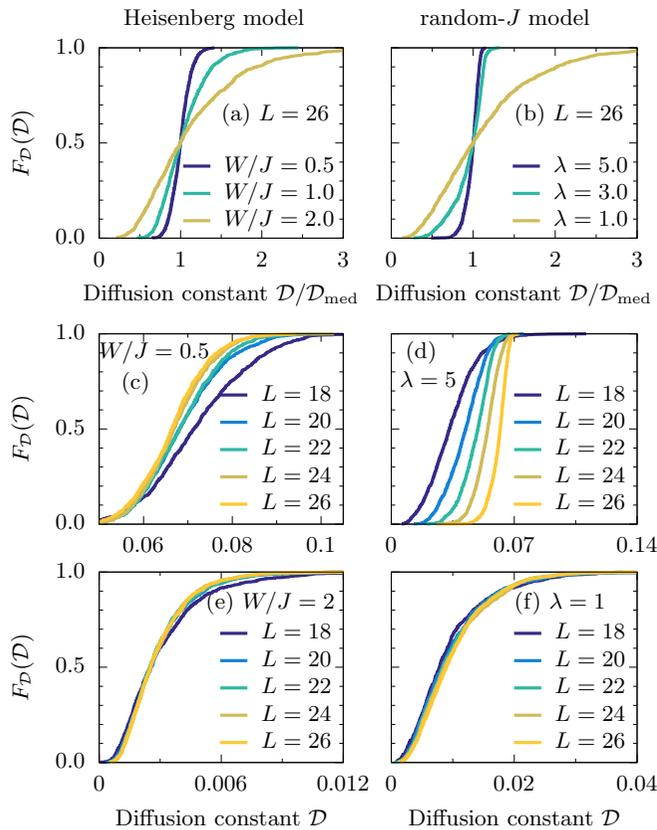
FIG. 4. Cumulative distribution functions  $F_{\mathcal{D}}(\mathcal{D})$  for various disorder strengths ( $W$ ) and system sizes ( $L$ ) calculated in the ergodic regimes of the random-field Heisenberg model (left column) and the random- $J$  Heisenberg model with  $f_J(J) = \lambda J^{\lambda-1}$  distribution (right column).  $\mathcal{D}$  in (a) and (b) are normalized by the median  $\mathcal{D}_{\text{med}}$ . Results are obtained from  $N_r = 10^3$  disordered samples.
