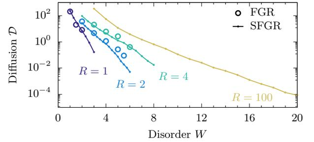
FIG. 1. Diffusion constant  $\mathcal{D}$  obtained from the rate equations with the Fermi golden rule (FGR) for  $L = 200$  and simplified FGR (SFGR, see text for details) for  $N = LR = 10^4$  with various numbers of legs  $R$  up to a 2D system for  $R \gg 1$ .
