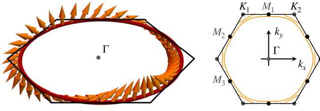
FIG. 9. d -wave spin Pomeranchuk order. Left panel: The order parameter of the d -wave spin Pomeranchuk order winds twice around the Fermi surface. Right panel: Diagonalization leads to a Zeeman-like term without net magnetization which splits the Fermi surface.
