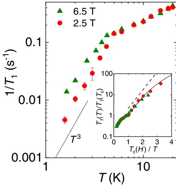
FIG. 3. Temperature dependence of  $1/T_1$ . Dotted line is a  $T^3$  dependence. The inset shows an Arrhenius plot of  $T_1(T)/T_1(T_c)$  vs  $T_c(H)/T$ . Solid curve is the calculation results assuming a two-dimensional  $d$ -wave SC gap and  $2\Delta_0(0)/k_B T_c \sim 4$  using Eq. (3). Broken line is an exponential dependence indicating fully gapped superconductivity.
