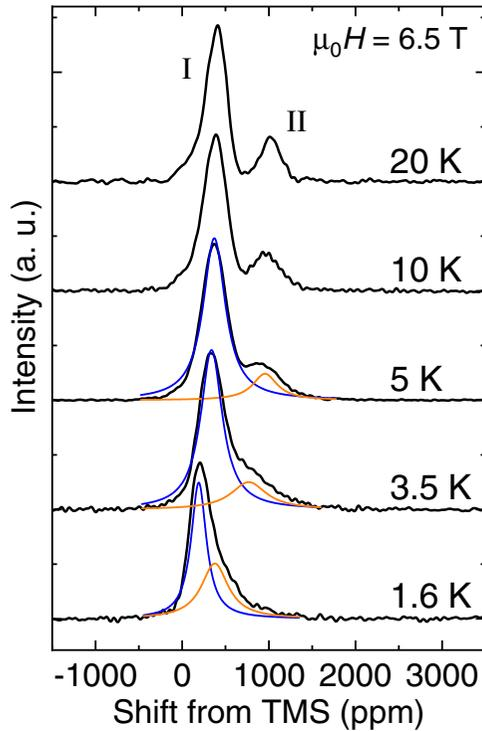
FIG. 1. NMR spectra of  $\lambda$ -(BETS) $_2$ GaCl $_4$  at several temperatures in a 6.5 T field parallel to the conduction plane. Blue and yellow lines are fitting curves using Lorentzian functions.
