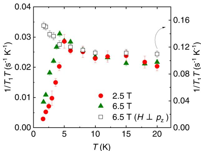
FIG. 4. Temperature dependence of  $1/T_1 T$  for  $\mu_0 H$  parallel to the conduction plane (left axis) and for  $\mu_0 H$  perpendicular to the  $p_z$  orbital of BETS molecule (right axis) [21].
