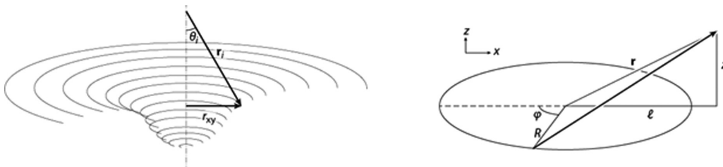
FIG. 6. Coordinate system as used in calculating electric field produced by surface electrons. Also shown (right) is the parameter for calculating field produced by an electron ring.
