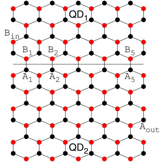
FIG. 3. Zero transmission in graphene:  $\mathbf{t}_{A_{\text{out}}, B_{\text{in}}}(0) = 0$  for all  $B_{\text{in}} \in QD_1$  and  $A_{\text{out}} \in QD_2$  for any constriction  $\tau_c$ .
