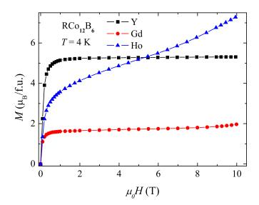
FIG. 2. Magnetization as a function of applied magnetic field for  $YCo_{12}B_6$ ,  $GdCo_{12}B_6$ , and  $HoCo_{12}B_6$  at T = 4 K.
