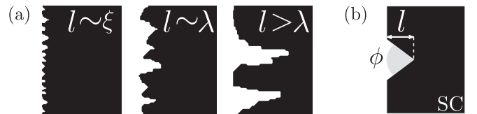
FIG. 4. (a) Examples of roughness profiles at the superconductor's edge tested in the simulations. In these three cases the profile is, going from left to right, comparable to the coherence length \xi , comparable to the penetration depth \lambda , and bigger than \lambda . (b) Model of a single dent: The depth is parametrized by l , while its sharpness by the angle \phi . The black color indicates the superconductor (SC).
