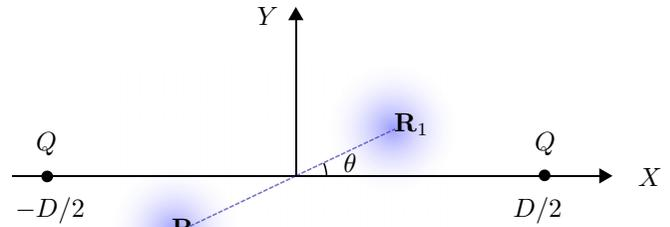
FIG. 1. Setup and coordinate system for a  $H_2$  molecule between point charges  $Q$  of equal sign, positioned at a distance  $D$  apart. The molecular axis, defined by nuclear coordinates  $\mathbf{R}_1$  and  $\mathbf{R}_2$ , forms a polar angle  $\theta$  with the  $X$  axis.
