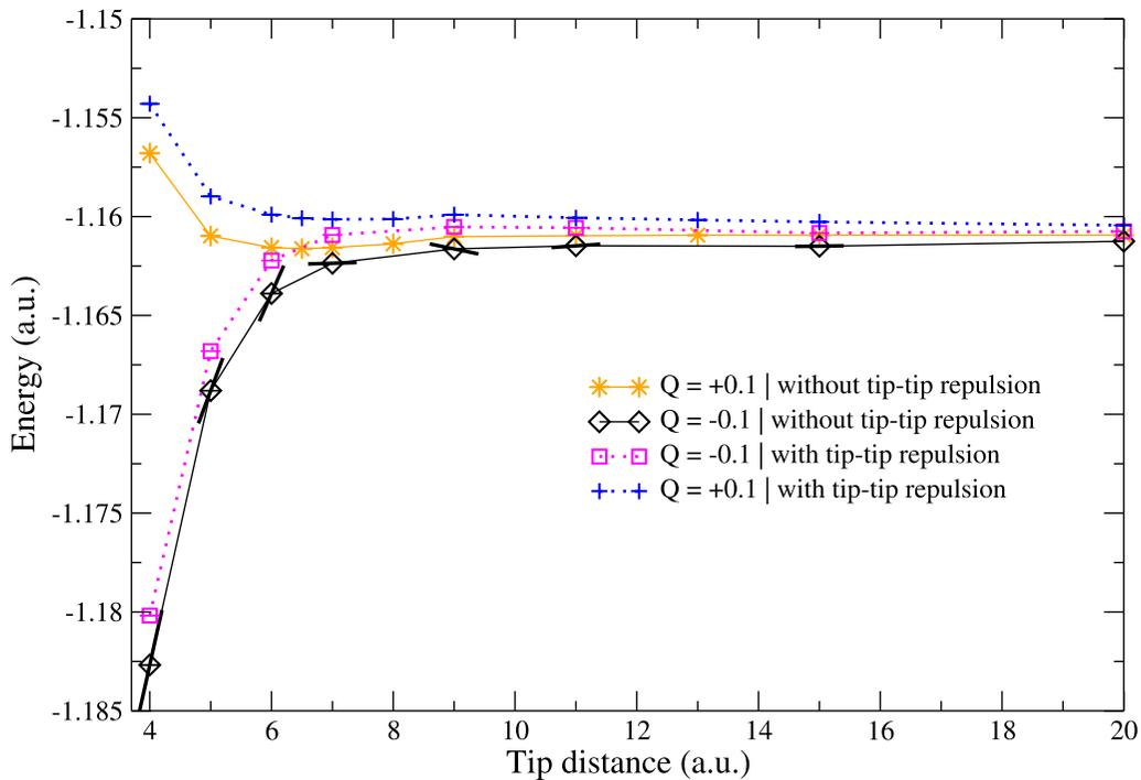
FIG. 3. Nonadiabatic ground states for axial symmetric nuclear wave-function ansatz plotted vs tip distance for both signs of tip charge:  $Q = -0.1$  a.u. without tip-tip potential (diamonds, solid) and with tip-tip potential (squares, broken);  $Q = +0.1$  a.u. without tip-tip potential (stars, solid) and with tip-tip potential (pluses, broken). Straight line sections at negative tip charge points represent tangents at those distances obtained from the virial equation; see, e.g., [21].
