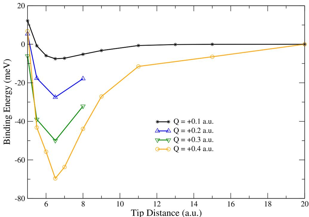
FIG. 4. Ground-state energy vs tip distance for equal positive tip charge of various amounts  $Q = 0.1, 0.2, 0.3$ , and  $0.4$  a.u. plotted by stars, up triangles, down triangles, and circles, respectively.
