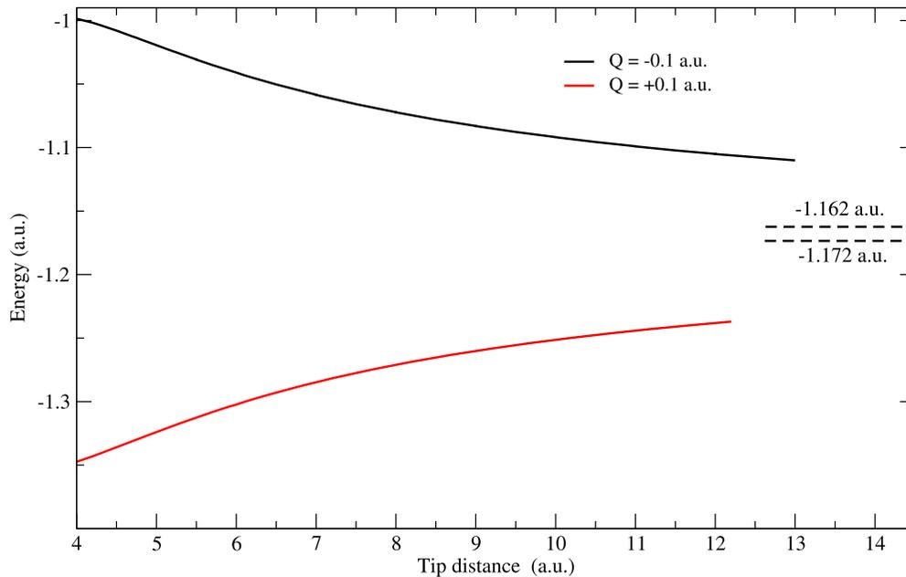
FIG. 2. Sampled adiabatic ground-state energy for PES with varying tip distance and both signs of a fixed amount of equal tip charge  $Q = -0.1$  a.u., upper curve (black), and  $Q = +0.1$  a.u., lower curve (red); the values obtained here for the free molecule, adiabatic (lower value) and nonadiabatic (upper value), are indicated at the right-hand side ordinate with dashed lines, which might be compared with  $E = -1.17448(2)$  a.u. of Tubman *et al.* [19]
