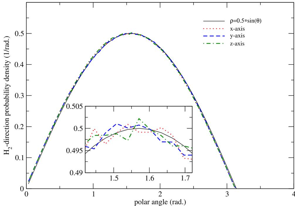
FIG. 6. Isolated ( $Q = 0$ )  $H_2$  molecule: Probability density of polar angles of  $H_2$  axis with respect to  $X$ ,  $Y$ , and  $Z$  axes sampled in full three-dimensional space; amplified resolution shown by the inset.
