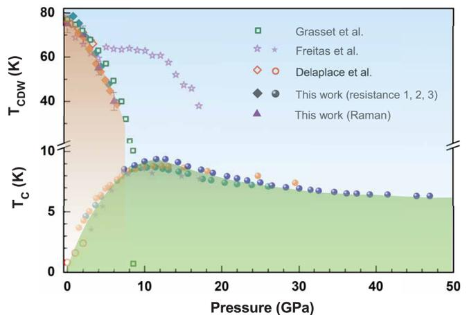
FIG. 5. The phase diagram of 2H-TaS<sub>2</sub>. Solid rhombuses represent  $T_{CDW}$  from the electrical resistivity measurements and the solid circles correspond to  $T_c$ ; the three independent runs were marked by different colors. Triangles denote  $T_{CDW}$  from Raman-scattering measurements. The experimental data points from the work of Refs. [24,25,42] were taken for comparison.
