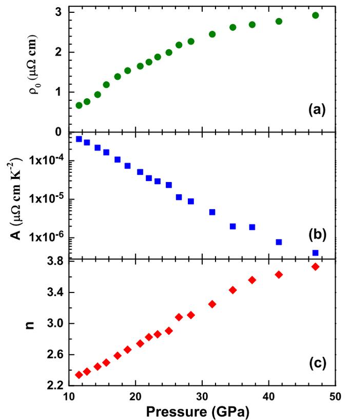
FIG. 6. Fitting parameters from the temperature-dependent resistivity in normal state of  $\text{TaS}_2$  at various pressures. (a) Pressure dependence of the residual resistivity  $\rho_0$ . (b) Plot of the prefactor  $A$  as a function of pressure. (c) The pressure-dependent resistivity exponent  $n$ .
