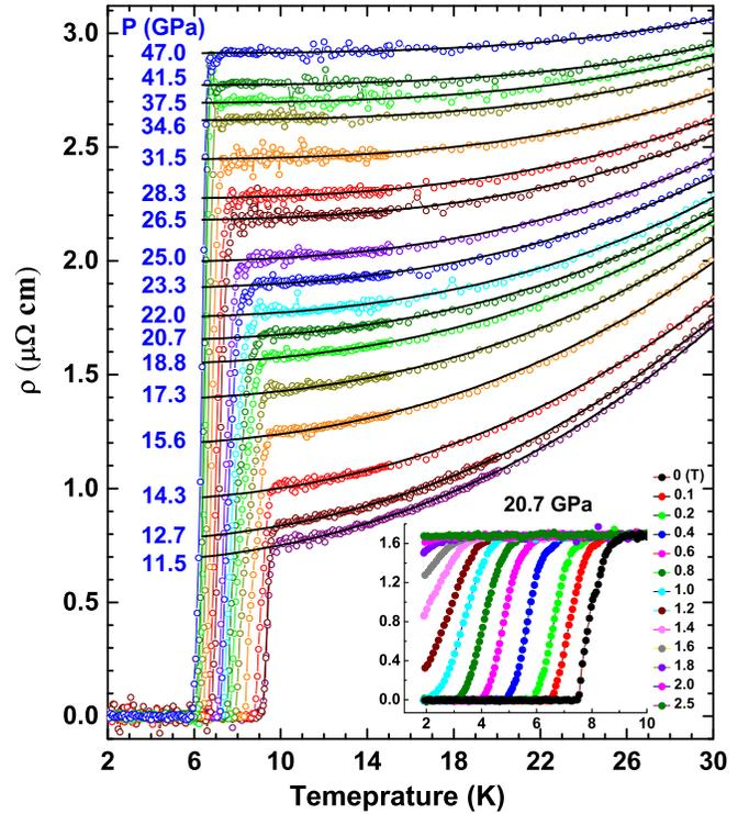
FIG. 4. Temperature dependence of the resistivity of TaS<sub>2</sub> upon further compression to 47 GPa. Raw data were signed with open circles. The black lines are fits to a standard resistivity formula:  $\rho(T) \simeq \rho_0 + AT^n$ . The inset shows the temperature-dependent resistivity at pressure of 20.7 GPa with the applied magnetic fields.
