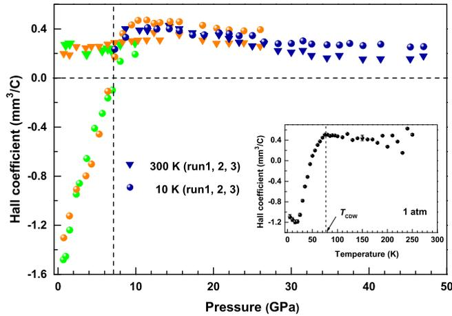
FIG. 3. The inverted triangles and solid circles denote the  $R_H$  values of TaS<sub>2</sub> at 300 K and 10 K, respectively. The vertical dashed line indicates the CDW transition. Inset: temperature dependence of  $R_H$  values for TaS<sub>2</sub> at ambient pressure.
