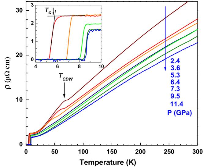
FIG. 2. Electrical resistivity of TaS<sub>2</sub> as a function of temperature at pressures up to 11.4 GPa,  $T_{CDW}$  is marked by an arrow. The inset shows superconducting transition within an enlarged region at low temperature and the criterion for determining  $T_c$ .
