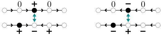
FIG. 6. Hopping of defects. To maintain the constraints, when a defect hops it has to flip a bond spin to its right, making its dynamics asymmetrical. In the original variables, this process is equivalent to emitting/absorbing a dipole from the right .
