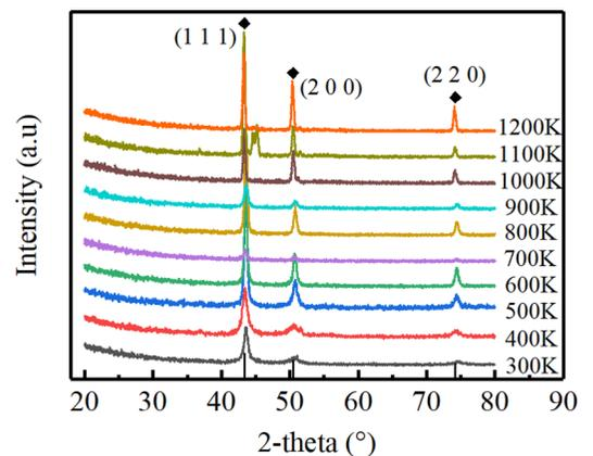
FIG. 7. X-ray diffraction pattern of Cu films annealed at different temperature from 300 to 1200 K. All the diffraction patterns have three diffraction peaks at  $43.4^\circ$ ,  $50.5^\circ$ , and  $74.2^\circ$ , corresponding to (111), (200), and (220) of Cu (ICSD-53247). With the annealing temperature increasing, both the 111, 200, and 220 peaks have exhibited obvious dynamic changes, which indicate the evolution of crystal structures in the Cu films.
