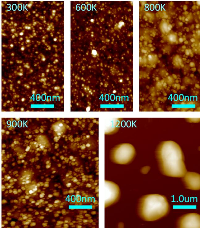
FIG. 6. Surface morphology of Cu films annealed at 300, 600, 800, 900, and 1200 K reported by AFM. All the micrographs are shown at the same scale of 500 nm. With the annealing temperature increasing, the Cu particles coalesce gradually to larger clusters. At the annealing temperature above 900 K, the islands or hillock are formed and separated.
