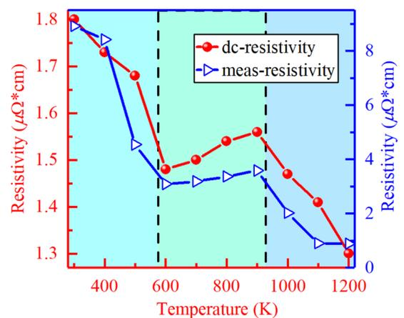
FIG. 11. dc resistivity obtained from fitting procedures and layer resistivity measured via four-probe method.
