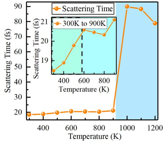
FIG. 12. Scattering time of conduction electrons at each annealed Cu film.
