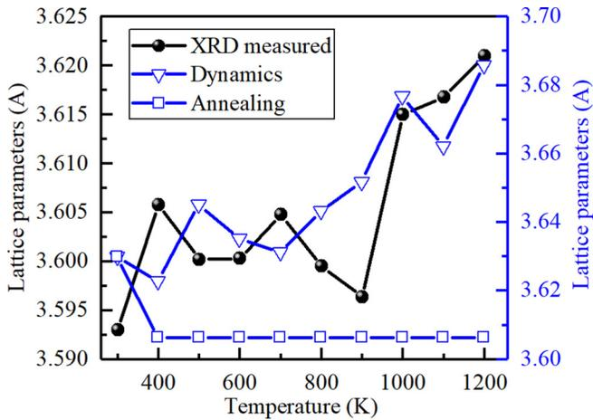
FIG. 9. The average lattice parameters obtained by XRD, thermal dynamics simulations, and annealing dynamics simulations. Both the thermal dynamics simulations and annealing dynamics simulations are carried out based on molecular dynamics.
