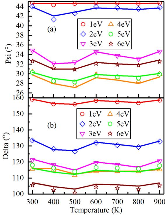
FIG. 2. Fitting results of  $\psi$  and  $\Delta$  for Cu films annealed at temperature from 300 to 900 K at the incident angle of  $60^\circ$ . (a) Fitting results of  $\psi$ ; (b) Fitting results of  $\Delta$ . Circles represent the measurement values, while solid lines stand for the calculated values. Both  $\psi$  and  $\Delta$  exhibit a transition temperature at 600 K, at which the variation tendency of both  $\psi$  and  $\Delta$  will change.
