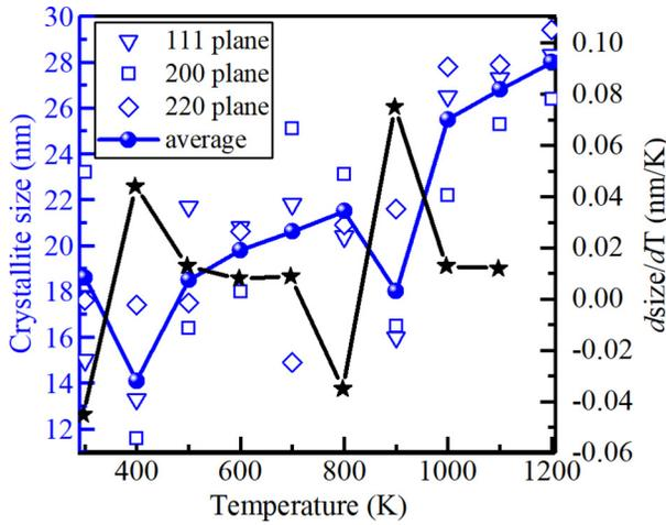
FIG. 8. The crystallite sizes in the (111), (200), and (220) plane obtained by XRD, the average crystallite size, and the thermal differential of average size. With the annealing temperature increasing from 300 to 1200 K, all the crystallite sizes exhibit the gradual upward trends.
