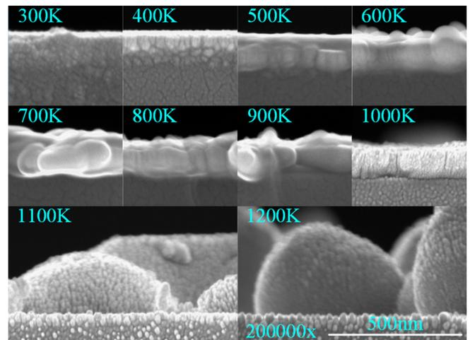
FIG. 10. Sectional view of Cu films annealed at different temperature. All the images are presented at the same scale and magnification. With increasing the annealing temperature, the Cu particles reaggregate on the lateral scale and eventually form island structure.
