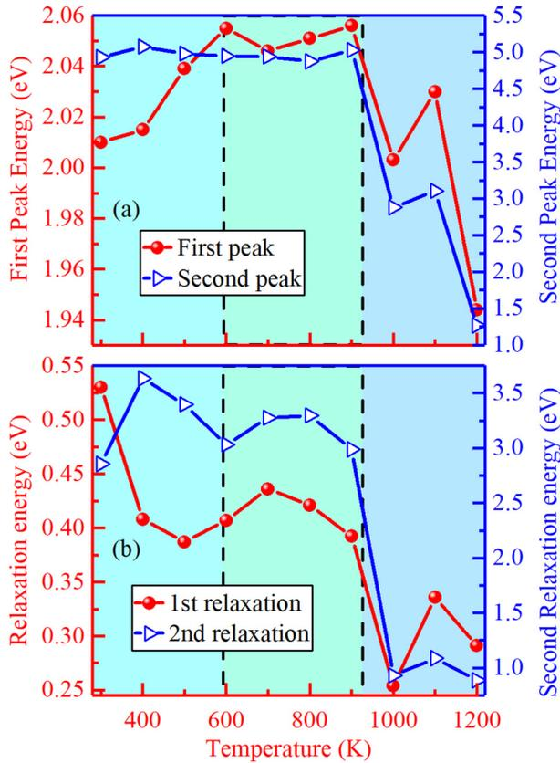
FIG. 13. Absorption peak energy and relaxation time of conduction electrons at each annealed Cu film.
