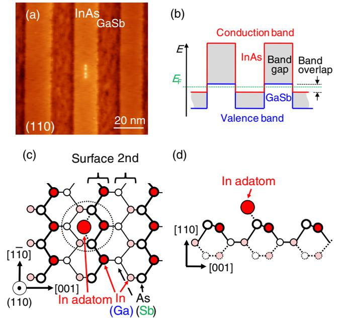
FIG. 1. (a) STM image of (110) cross-sectional surface of InAs(16 nm)/GaSb(16 nm) quantum structures with four manipulated adatoms on an InAs layer (sample bias voltage  $V = +1.0 \text{ V}$  and feedback tunneling current  $I = 200 \text{ pA}$ ). (b) Schematic energy band profile for InAs/GaSb quantum structures. (c) Stick-and-ball model for the (110)InAs (GaSb) surface with one manipulated adatom and (d) its cross section.
