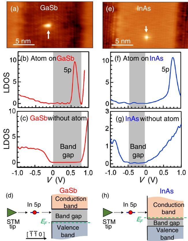
FIG. 4. (a) STM image of one adatom positioned at the center of a GaSb layer ( $V = 1.0$  V,  $I = 100$  pA). (b) and (c) Tunneling spectra measured on the adatom and on the GaSb layer without an adatom. (d) Schematic energy diagram of the tunneling process on the GaSb layer via the positioned adatom. For clarity, the potential modulation due to the positively charged adatom discussed in a later part is not shown. (e)–(h) Corresponding panels for an InAs layer.
