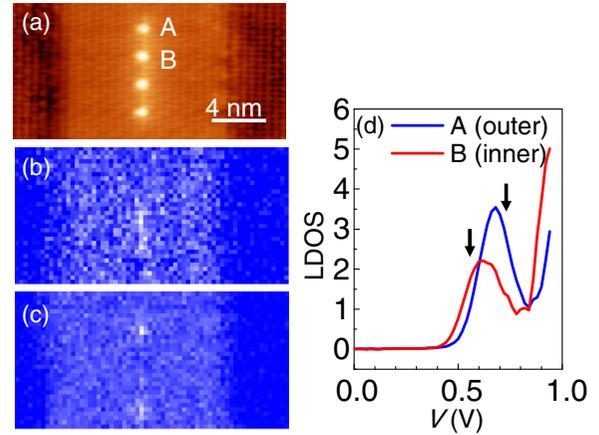
FIG. 3. (a) STM image of four assembled In adatoms on an InAs QW ( $V = 1.0$  V,  $I = 200$  pA). The distance between the adjacent adatoms is  $\frac{5}{\sqrt{2}}a$ , where  $a = 0.606$  nm is the lattice constant. (b) and (c) LDOS maps over the area in (a) at  $V = 0.57$  and  $0.73$  V [corresponding to the arrows in (d)], respectively. (d) LDOS spectra as a function of  $V$  measured on adatoms “A” and “B” in (a).
