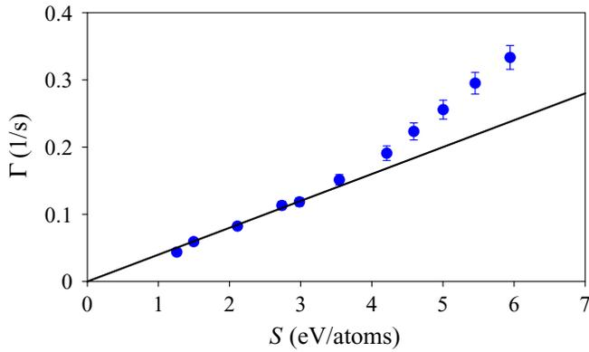
FIG. 4.  $\Gamma$  as a function of average dose rate  $S$  in  $(\text{Rb}_2\text{O})_{30}(\text{B}_2\text{O}_3)_{70}$  measured at  $q_{\text{max}}$ . The blue solid circles indicate a measurement series of different combinations of absorbers, while the line corresponds to a strictly linear proportionality.
