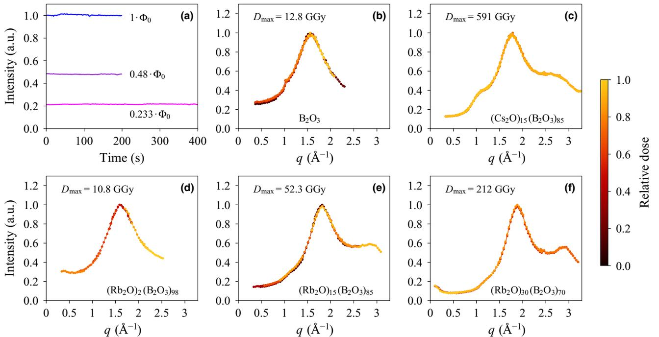
FIG. 2. Quantification of beam damage under irradiation: (a) shows the time evolution of the intensity  $I(t)$  for  $(\text{Rb}_2\text{O})_{15}(\text{B}_2\text{O}_3)_{85}$  measured under different incoming  $\Phi_{\text{in}}$  at  $q_{\text{max}}$ . (b)–(f) show the evolution of  $I(q)$  with accumulated dose for the various systems, with the dose relative to its final value encoded in the color of the curves.
