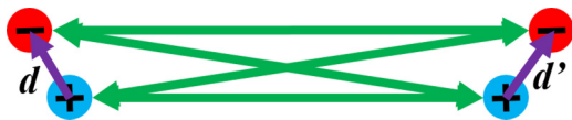
FIG. 1. Diagram of the two interacting excitons. The green arrows depict the Coulomb coupling between the two excitons that generates the interaction energy, and the purple arrows depict the hole-to-electron vectors for the excitons ( \mathbf{d} and \mathbf{d}' , respectively). Note that the interexciton spacing is much greater than the size of each exciton.
