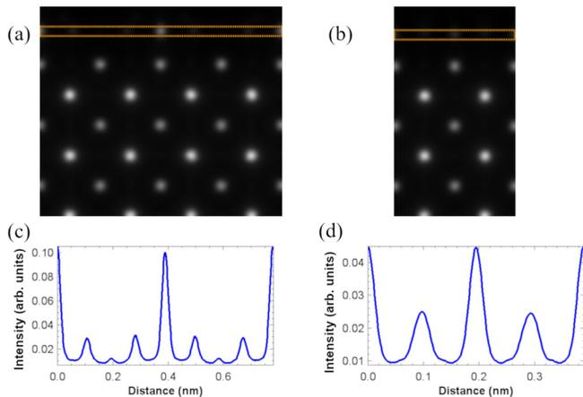
FIG. 7. Simulated HAADF images of the view down the  $a$  and  $b$  crystallographic directions of the  $(4 \times 2)$  surface reconstruction of Ref. [55] [(a) and (b), respectively, with the corresponding line profiles appearing in (c) and (d)]. Again, the view along  $b$  agrees somewhat with the FeSe/STO interface, but the same caveats apply as in the  $(2 \times 1)$  structure.
