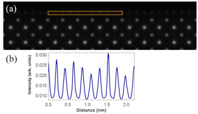
FIG. 8. (a) Simulated HAADF images of the  $R33.7^\circ$  ( $\sqrt{13} \times \sqrt{13}$ ) surface reconstruction of Ref. [56]. (b) Line profile across the second Ti-O layer. In this case, although there are similarities between the appearance of this layer and that seen experimentally in the FeSe/STO interface, neither the periodicity nor the magnitude of the Ti column intensities agree with the latter.
