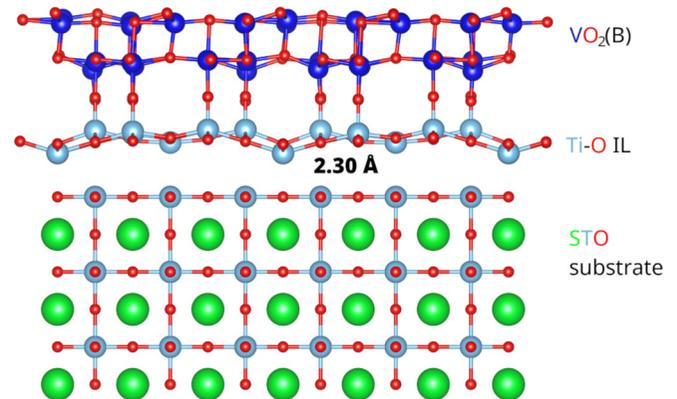
FIG. 9. Relaxed structure of the VO<sub>2</sub>(B)/Ti<sub>1+x</sub>O<sub>2</sub>/SrTiO<sub>3</sub> interface, based on the experimental results of Ref. [33]. The buckling of the interfacial layer is more pronounced here, as the Ti<sub>1.5</sub>O<sub>2</sub> layer partially conforms to the structure of the layer above. Unlike in FeSe/STO, the interfacial layer forms chemical bonds with VO<sub>2</sub>, allowing the monoclinic bronze phase to grow epitaxially on cubic STO.
