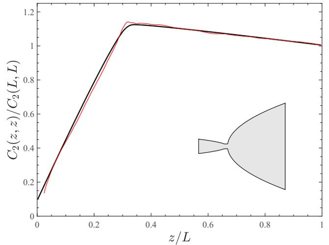
FIG. 4. Thick solid line in the main plot depicts  $C_2(z, z)$  in a two-dimensional expanding disordered waveguide defined by Eq. (23). Thin line is the result of numerical simulation. The inset plots the shape of the considered waveguide.
