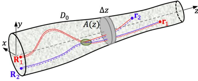
FIG. 1. Schematic depiction of a disordered waveguide with varying diameter. In diagrammatic description of wave transport, the long-range correlation between intensities at  $\mathbf{r}_1$  and  $\mathbf{r}_2$  arises when two propagation paths, described by the Green's function of diffusion equation, intersect allowing a swap of field amplitudes.
