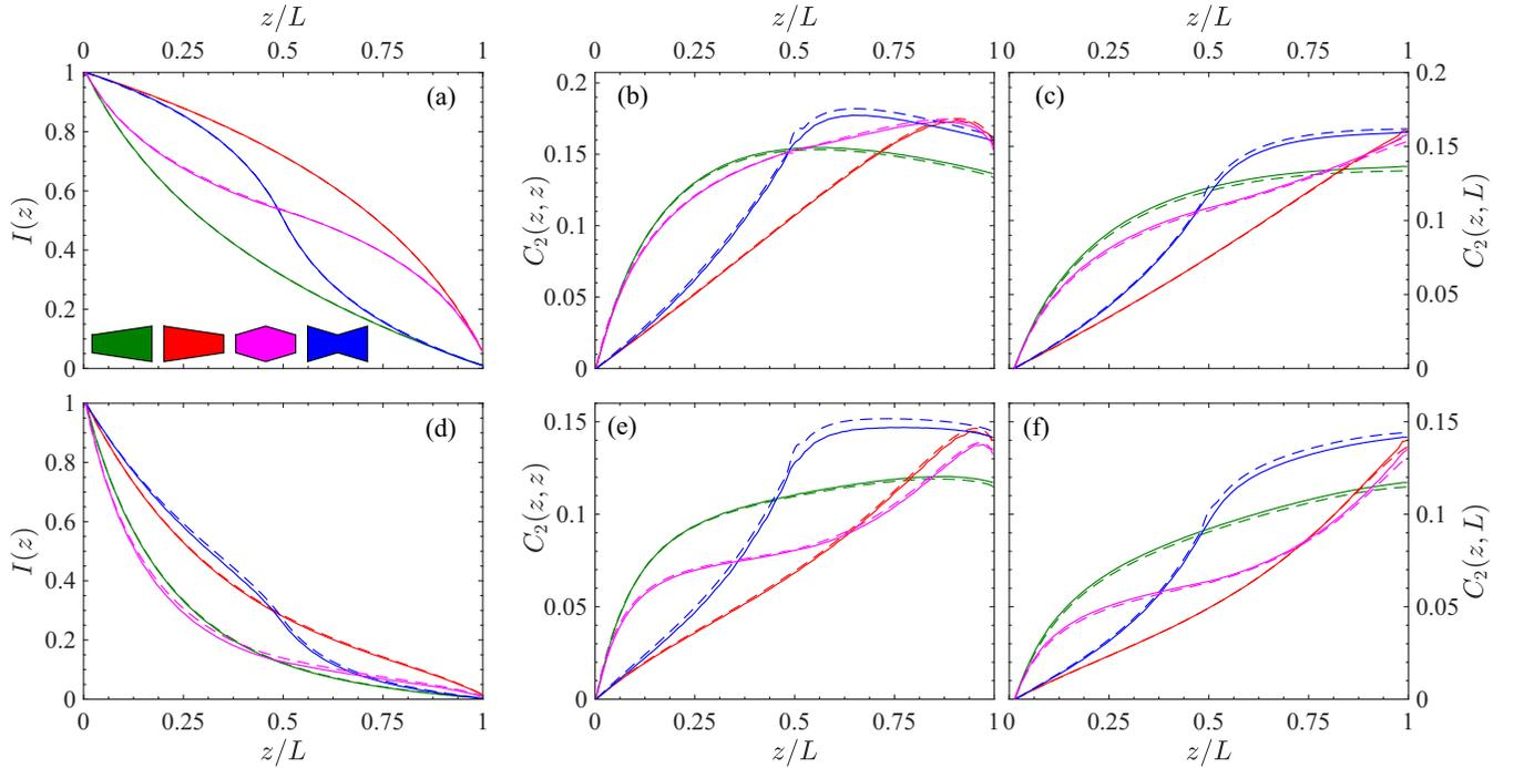
FIG. 2. Intensity and the long-range correlation computed using 2D calculations (solid lines) and projection to 1D technique (dashed lines). Line color corresponds to one of the four waveguide shapes depicted in the inset of panel (a). Passive/absorbing waveguides are shown in (a)–(c) and (d)–(f) respectively; see text for system parameters.
