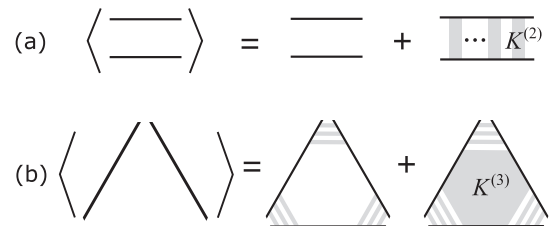
FIG. 9. Diagrammatic representation for the equations used to compute (a) K_i^{(2)} and (b) K_i^{(3)} under CPA. All the objects in the diagrams are local in space. The angle brackets denote disorder average over the random potential v_i . The stripes in (b) denote the ladder series of K_i^{(2)} (see Ref. [14] for more details).
