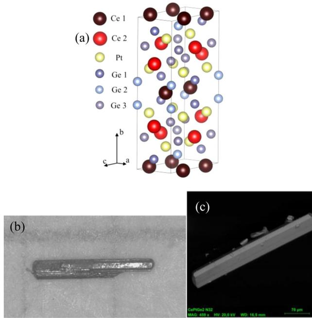
FIG. 1. (a) The crystal structure of  $\text{CePtGe}_2$ . (b) A single crystal of  $\text{CePtGe}_2$  grown under Bi flux. (c) Scanning electron microscopy image of a single crystal of  $\text{CePtGe}_2$  grown under Pb flux.
