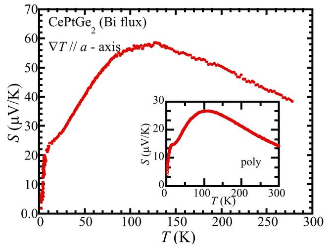
FIG. 6. Temperature dependence of the Seebeck coefficient for single-crystalline and polycrystalline (inset) CePtGe<sub>2</sub>.
