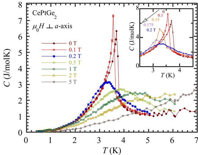
FIG. 4. Temperature dependence of specific heat for a single crystal of CePtGe<sub>2</sub>. The inset shows the expansion around  $T_N$ .
