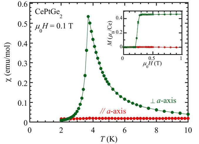
FIG. 3. Temperature dependence of  $\chi$  for single-crystalline CePtGe<sub>2</sub>. The inset shows the magnetic field dependence of magnetization at 2 K.
