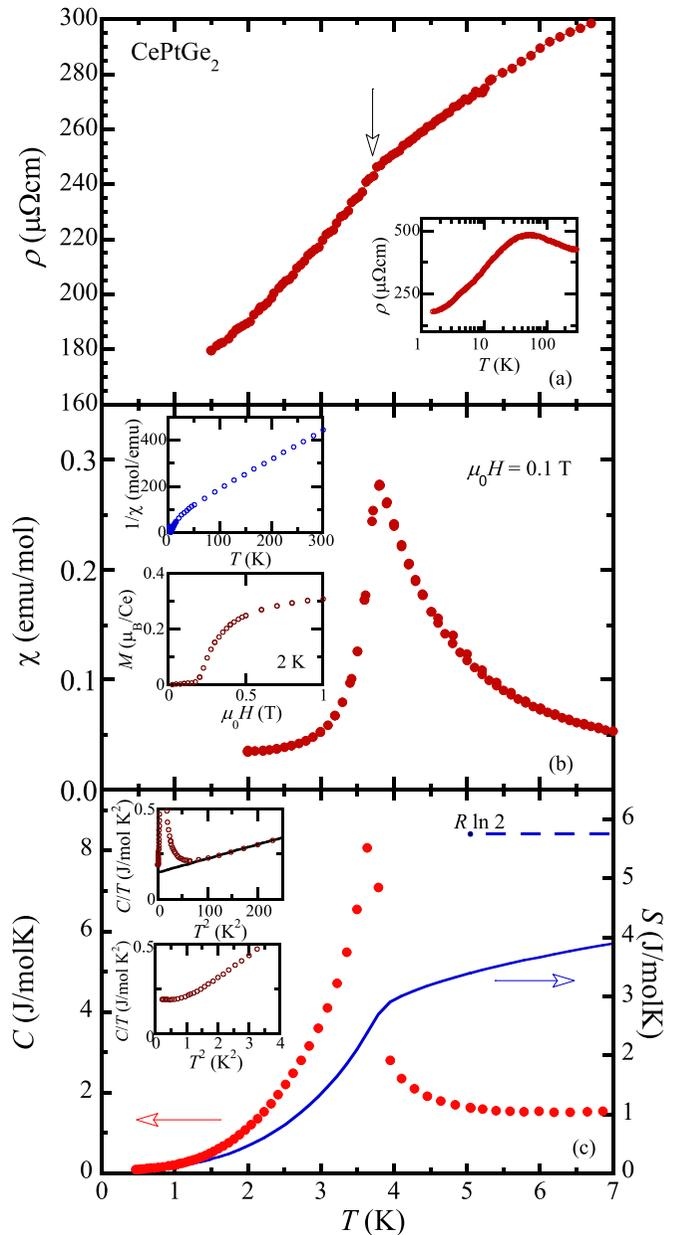
FIG. 2. (a) Resistivity of  $\text{CePtGe}_2$  in the low-temperature region. The inset shows the resistivity in the entire temperature range. (b) Susceptibility of  $\text{CePtGe}_2$  as a function of temperature. The insets show the inverse susceptibility and field dependence of magnetization. (c) Temperature dependence of specific heat and entropy for  $\text{CePtGe}_2$ . The insets show  $C/T$  versus  $T^2$  in the entire temperature range and in the low-temperature region.
