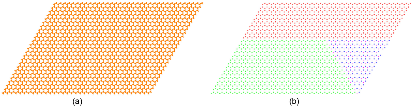
FIG. 5. Digital models assisting the two steps machining process. (a) Digital model assisting the waterjet cutting. (b) Digital model assisting the drilling machine. Holes in red (green) define the H^+ ( H^- ) topological phase and are blind, i.e., drilled for a height of h = 5.4 mm from the top (bottom) to the bottom (top) of the plate with a radius R = 1.75 mm. Holes in blue (violet) define the V^R ( V^l ) topological phase and are drilled through the plate thickness, with a radius of R = 1.75 ( r = 0.90 ) mm.
