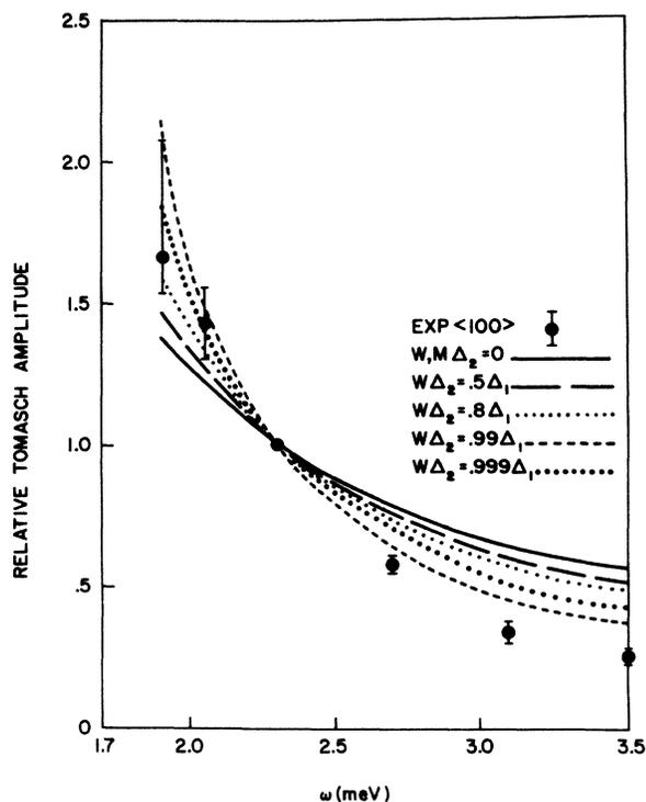
FIG. 4. Comparison of experimental Tomasch envelopes with theory for differing proximity contributions. For W,  $\Delta_2$  is the gap in silver,  $\Delta_1$  that in lead.
