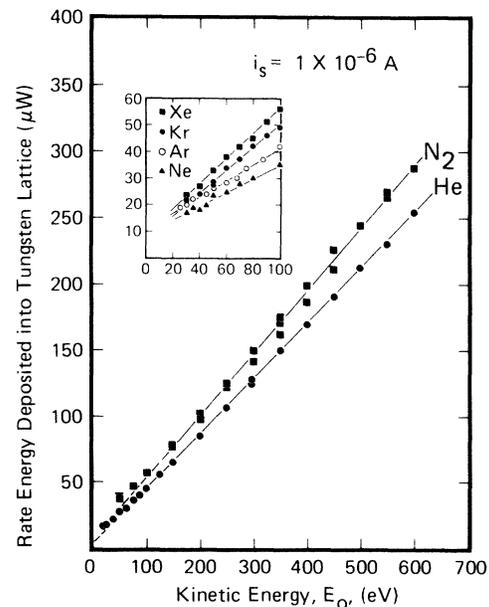
FIG. 8. Rate of energy deposition vs the initial kinetic energy of the ions. The data have not been corrected for secondary emission or pressure.  $i_s$  is the bombarding-ion current.
