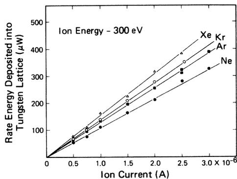
FIG. 5. Rate of energy deposition vs ion current. The data are not corrected for pressure or secondary-electron emission.
