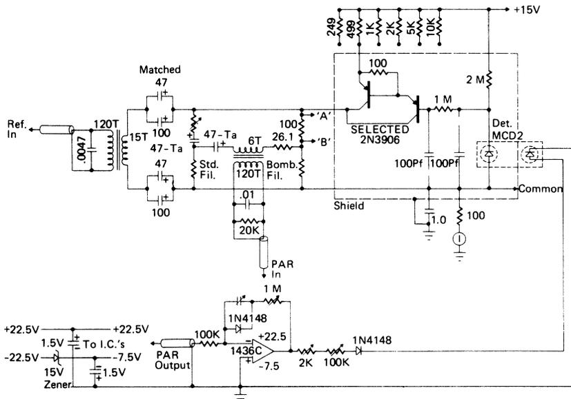
FIG. 2. Schematic of control electronics. Transformers wound on Ferroxcube Toroid K300-502/3E with No. 24 wire, 2N3906's selected for high beta at 100- $\mu$ A collector current.
