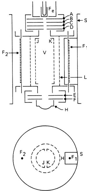
FIG. 1. Schematic diagram of experimental tube.  $F_1$  is the standard filament which was shielded from the ions.
