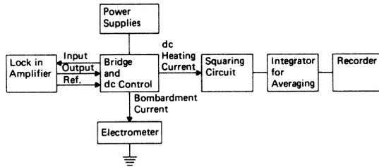
FIG. 4. Block diagram of electronics.
