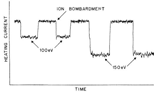
FIG. 3. Heating current vs time. The sharp drop in the heating current occurs when ion bombardment is initiated.
