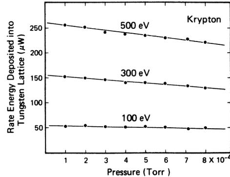
FIG. 6. Rate of energy deposition vs pressure.
