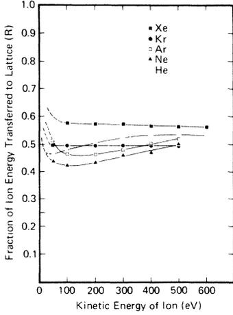
FIG. 9. Fraction of energy transferred to lattice vs initial kinetic energy. The data have been corrected for secondary emission and to zero pressure,  $R = E_{\text{tot}}/E_0 + E_T$ .
