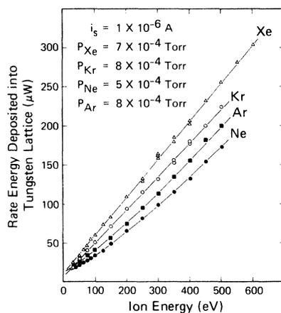
FIG. 7. Rate of energy deposition vs the initial kinetic energy of the ions. The data have not been corrected for secondary emission or pressure.  $i_s$  is the bombarding-ion current.
