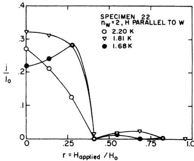
FIG. 10. Effect of a field on a zero-field vortex mode. The field is parallel to the presumed direction of propagation of the vortex and should not excite the corresponding Fiske mode. (Applying a field in the perpendicular direction gives similar results, but the behavior is confused by the appearance of the Fiske mode).
