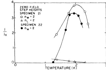
FIG. 9. Some zero-field step heights, divided by the supercurrent at the same temperature, against temperature. The solid lines are intended merely to be suggestive. The open and solid circles represent "large" steps, and the triangular points are for a "small" step with voltage beyond cutoff. For the circles, note the qualitative similarity with Fiske-mode behavior (as illustrated in Fig. 4).
