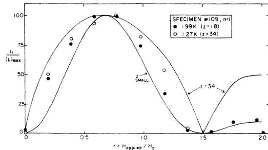
FIG. 1. Step height against applied field for the  $n=1$  Fiske mode of junction 109 at two temperatures. The data and theoretical curves are normalized by dividing by the maximum value, so that each has a peak value of unity. The theoretical curves and  $z$  values were determined from Kulik's theory, as described in the text.  $H_0$  is the field that gives one flux quantum in the junction. Note that the "small  $z$ " and "z=3.4" curves differ little for  $r < 1.5$ .
