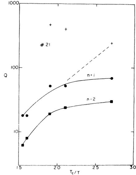
FIG. 5. Quality factor  $Q$  against  $T_c/T$  for the Fiske modes of junction 21. The crosses and dashed line show alternate choices for  $n=1$ . This ambiguity is explained in the text. The solid lines are intended merely to be suggestive.
