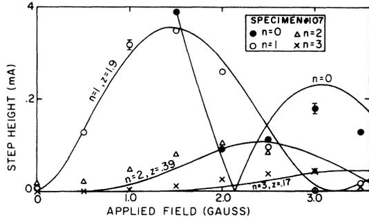
FIG. 3. Current step height against field for the zero-voltage supercurrent ( $n=0$ ) and the Fiske modes ( $n=1, 2, 3$ ) of junction 107 at 2.03 K. The solid lines and corresponding  $z$  values were determined using Kulik's theory. The  $z$  value was chosen so that the theoretical curve would have the same maximum step height as the data.
