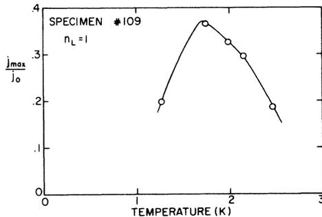
FIG. 4. Temperature dependence of the  $n_L=1$  Fiske mode of junction 109.  $j_{\max}$  is the height of the step at whatever applied field maximizes it, and  $j_0$  is the zero-field supercurrent density at the same temperature. The rather sharp peak near 1.7 K ( $T/T_c=0.5$ ) corresponds to the peak in Fig. 2. The solid line is intended merely to be suggestive.
