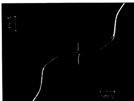
FIG. 5. V - I characteristic for a Sn-Sn x O y -In Josephson junction at T=1.21 K. Horiz. scale: 0.5 mV/div.; vert.: 1 mA/div.
