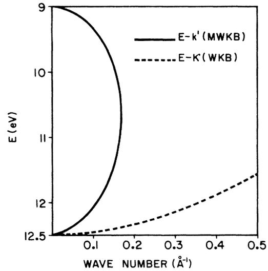
FIG. 4. Dispersion relation within the energy gap.  $E-k'$  characteristics of the insulator from band structure, Eq. (10): full line;  $E-k$  relation from usual WKB approximation, Eq. (22): dashed line.
