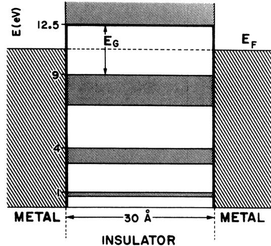
FIG. 2. Energy-band relations at the metal-insulator-metal interfaces with no bias applied. The band structure of the insulator, calculated with the parameters given in the text, is indicated with the dashed regions corresponding to allowed energy bands.  $E_F$  is the Fermi energy of the metal and  $E_G$  is the energy gap of the insulator. The heavy line represents the square potential barrier used in the trapezoidal model.
