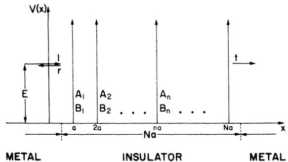
FIG. 1. Model potential for a symmetric MIM structure. The vertical arrows denote equally spaced  $\delta$ -type potentials. The horizontal arrows denote an incoming electron from the left metal with energy  $E$  and amplitude 1 which is reflected with amplitude  $r$  and transmitted through the insulator with amplitude  $t$ .  $A_n$  and  $B_n$  are the amplitudes of the forward and backward plane waves, respectively, in the interval  $n$ .
