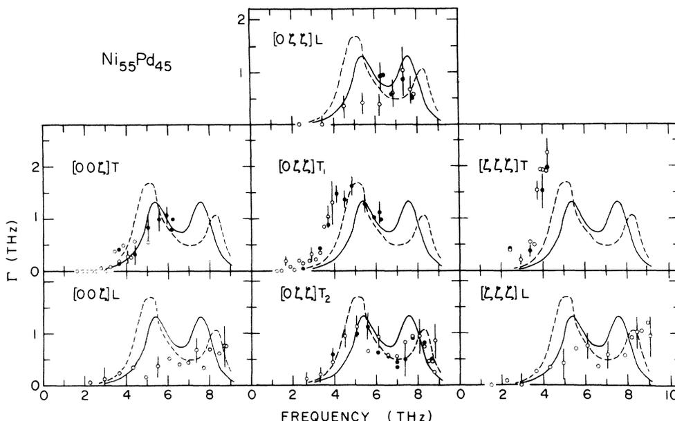
FIG. 4. Natural widths for  $\text{Ni}_{55}\text{Pd}_{45}$  plotted against reference-lattice (Ni) frequency for each branch. The solid lines represent the predictions of the self-consistent theory, and the dashed lines represent those of low-concentration theory.
