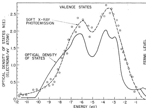
Fig. 14. Comparison of the ODS and the soft-x-ray photoemission results of Siegbahn *et al.* (Ref. 20). The x-ray results have been shifted to lower energy by 0.6 eV to obtain the best fit. (It is difficult to set the absolute zero of energy in the x-ray experiment.)
