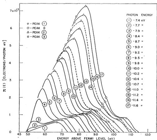
FIG. 5. A family of energy distribution curves (EDC's) for gold in the range  $7.4 \leq h\nu \leq 11.6$  eV. The EDC's have been normalized to yield. Peaks ①, ②, and ③ correspond to peaks in the valence ODS of Fig. 1. Peak D is due to a direct transition believed to originate near the  $L_2'$  symmetry point. These data were taken under good vacuum conditions.
