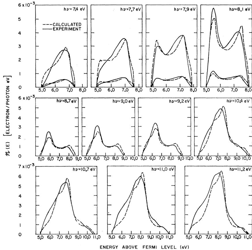
FIG. 11. Comparison of calculated and measured EDC's for  $7.4 \leq h\nu \leq 11.2$  eV. For  $7.4 \leq h\nu \leq 8.1$  eV, an enlarged set of curves is given by multiplying the absolute curves times 5. For additional curves see Ref. 9.
