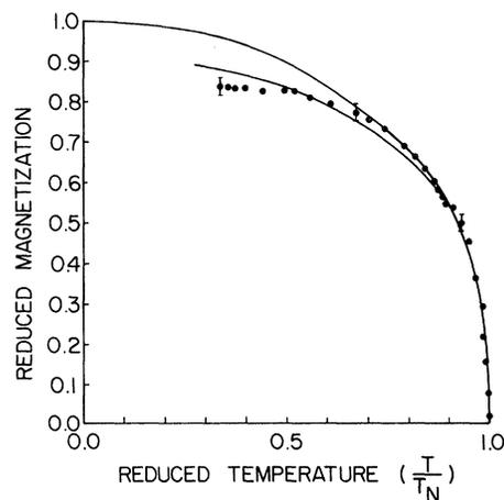
FIG. 1. Temperature dependence of the weak ferromagnetic moment of hematite. The upper curve represents the normalized temperature dependence of the sublattice magnetization,  $M/M_0$ , the dots are the experimental data  $m/m_0$ , while the lower curve is calculated from Eq. (6).
