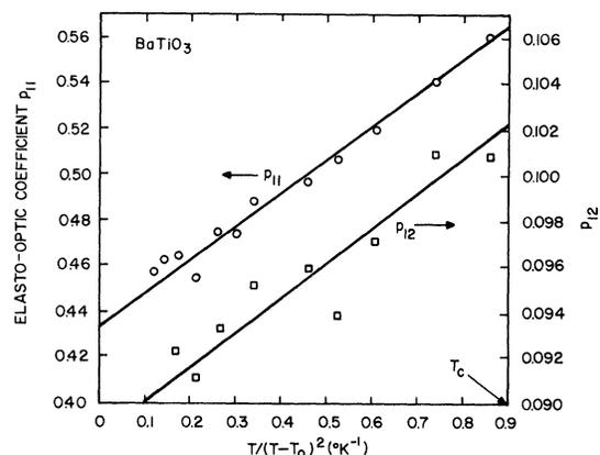
FIG. 2. Dependence of  $p_{11}$  and  $p_{12}$  elasto-optic coefficients on the quantity  $T / (T - T_0)^2$  [see Eq. (7)]. The Curie-Weiss temperature in this sample is  $T_0 = 110^\circ\text{C}$  (see Ref. 16).
