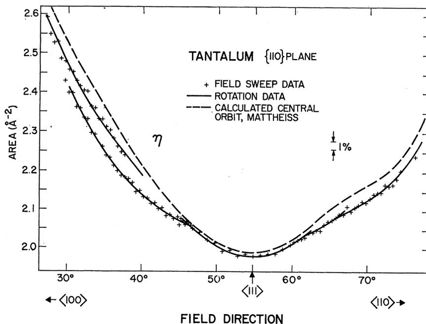
FIG. 5. Extremal Fermi-surface areas in tantalum as a function of angle in the  $(1\bar{1}0)$  plane for the  $H$  intersection of the jungle gym. Discontinuities in rotation data are real and probably result from protrusions on the surface.
