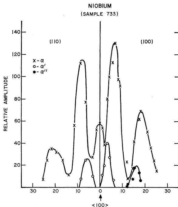
FIG. 6. Amplitude variation of  $dT/dH$  with angle in the  $(1\bar{1}0)$  and  $(001)$  planes for  $\alpha$ ,  $\alpha'$ , and  $\alpha''$  frequencies. The lines connecting the points serve only to distinguish the  $\alpha$ ,  $\alpha'$ , and  $\alpha''$  data.
