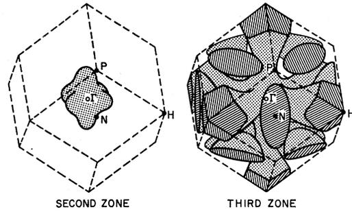
FIG. 1. Calculated Fermi surface of niobium; (a) closed second-zone hole surface centered at  $\Gamma$ , (b) third-zone hole surfaces including the open jungle-gym surface and the set of six distorted ellipsoids which are indexed according to the numbers in the figure.
