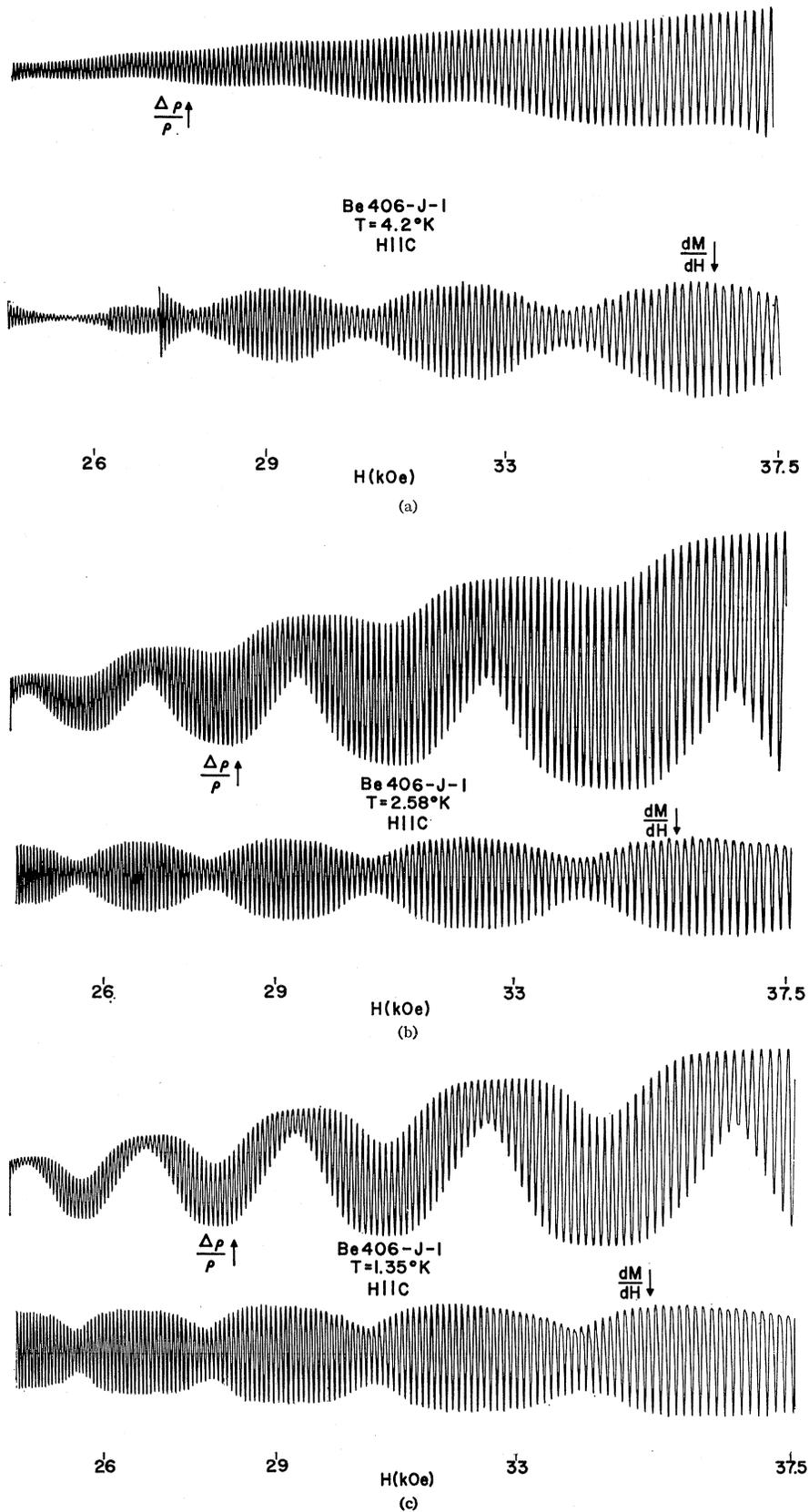
FIG. 4. Field dependence of the magnetoresistance ( $\Delta\rho/\rho$ ) and differential magnetic susceptibility ( $dM/dH$ ) (a)  $T = 4.2^\circ\text{K}$ ; (b)  $T = 2.58^\circ\text{K}$ ; (c)  $T = 1.35^\circ\text{K}$ .
