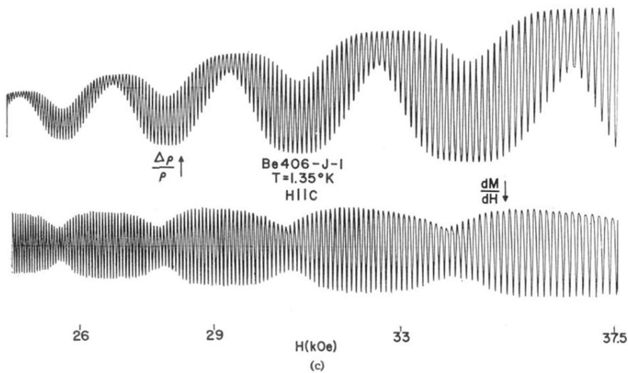
FIG. 4. Field dependence of the magnetoresistance ( $\Delta\rho/\rho$ ) and differential magnetic susceptibility ( $dM/dH$ ) (a)  $T = 4.2^\circ\text{K}$ ; (b)  $T = 2.58^\circ\text{K}$ ; (c)  $T = 1.35^\circ\text{K}$ .
