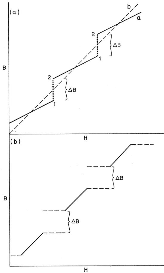
FIG. 5. (a)  $B$  versus  $H$ , curve  $a$ : in regime of magnetic interactions showing discontinuity in  $B$ ; curve  $b$ :  $B=H$ . (b)  $B$  versus  $H$  for disk shaped sample ( $L=1$ ). Magnetic domains form in dashed regions of curve.
