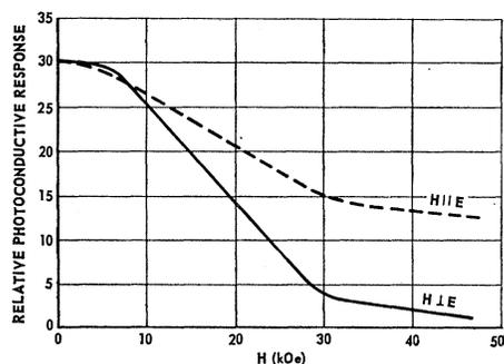
FIG. 5. Photoconductive response of gallium-doped germanium at 119  $\mu\text{m}$  in transverse and longitudinal magnetic fields.
