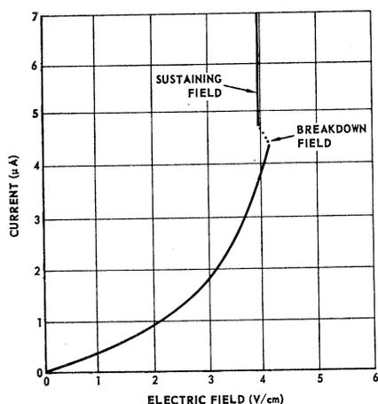
FIG. 2. Current-electric-field characteristic for Ge:Ga at 4.2°K.
